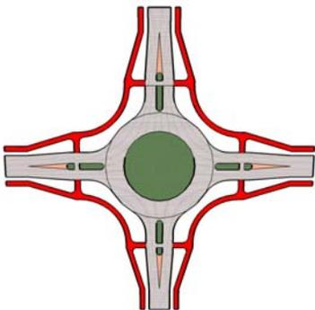
Figure 4 - - Roundabout with grade-separated cycle paths
