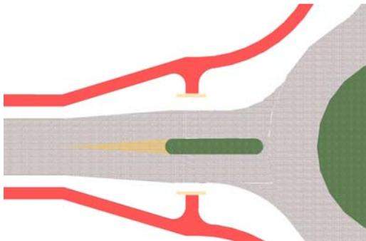
A second possible solution are cycle lanes next to the carriageway, but still within the roundabout (figure 2, see also picture 1). Those lanes are constructed on the outside of the roundabout, around the carriageway. They are visually recognizable for all road users. They may be separated from the roadway by a road marking and/or a small physical element or a slight elevation. They may also be constructed with a different pavement or
